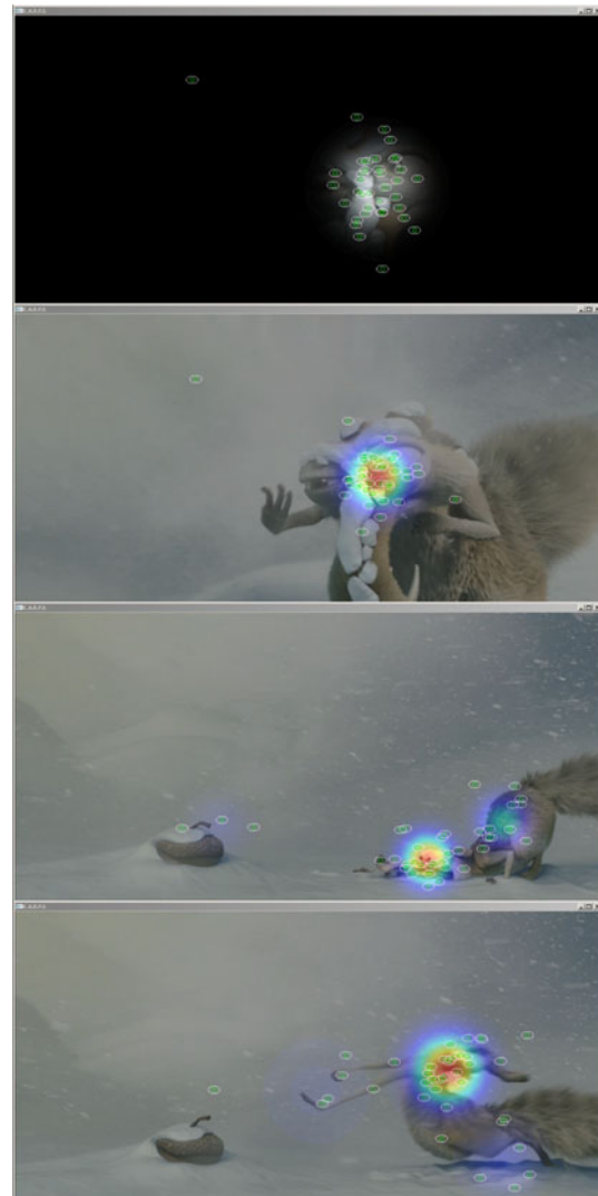
Fig. 9 Example stills from clustering binocular eye tracking data on video 16. Blue values correspond to 0.0 and red to 1.0. The first example still uses the values of the GMM as an alpha-map layer providing a ‘peek-through’ effect. Notice the robustness to noise given the large number of data samples in the first still (original movie image of Ice Age 3 Trailer Copyright Twentieth Century Fox)
